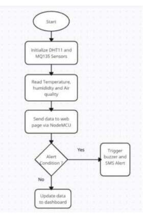
The flowchart depicts the operation of an Unpredictable Environmental Monitoring and Alert System using NodeMCU. The process starts with the initialization of the DHT11 and MQ135 sensors, which are tasked with sensing temperature, humidity, and air quality. After initialization, the system keeps reading the environmental data from the sensors continuously.All the collected data is sent to our webpage using the NodeMCU for monitoring.
